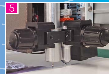
Dual tools for cutting and creasing simultaneously
