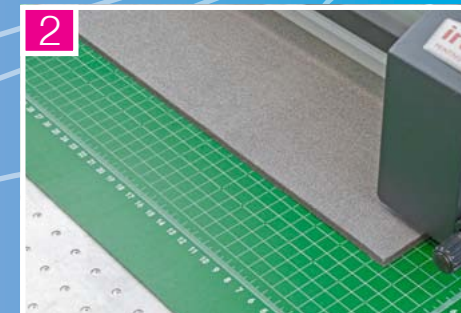
Vacuum suction system holds media during cutting
