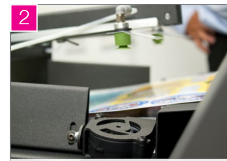
Air separation system
